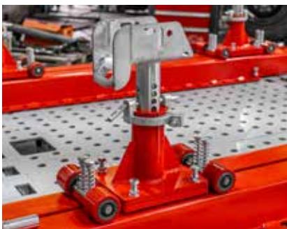
Special adapters fix any cab to mobile supports with carriages.
