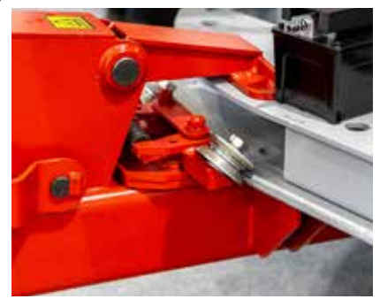
Original roller mechanism for easy movement. Fast and rigid fixation in one of 112 positions.
