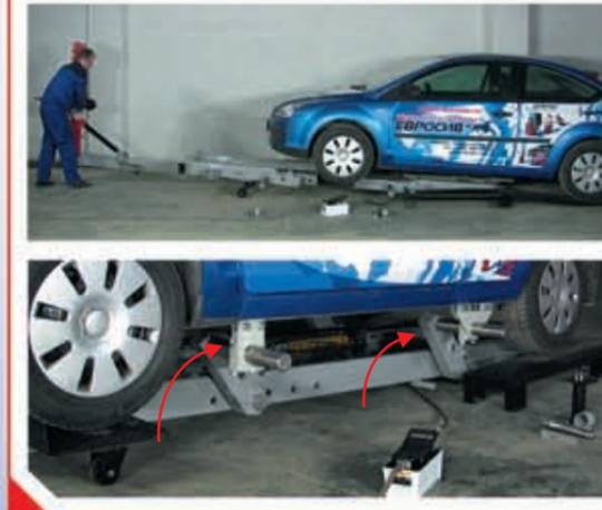
System is equipped with 2 and 3 hinges pulling device. Hydraulic power of each is 10 tons. 3-hinges pulling device offers more accurate pulling, no need to move it.
