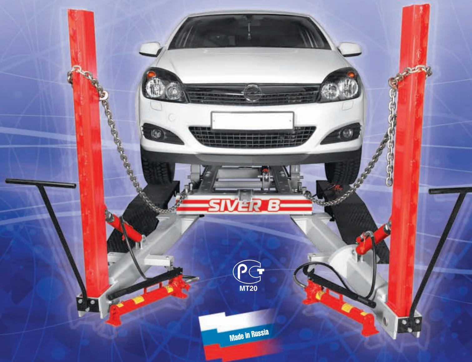
Pulling system **SIVER B** is intended for collision repair of damaged vehicles in weight up to 2000 kg. All equipment supplied with Certificate of conformity to safety requirements. **SIVER B** features quality check, mobility, easy storage and reasonable price.
